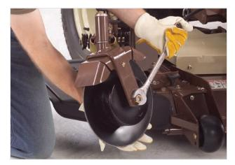
Reverse disc by removing one bolt to edge from the turf.
