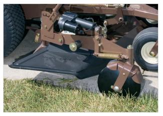
Edge-EZE<sup>™</sup> discharge shield allows you to blow debris off sidewalk into turf.
