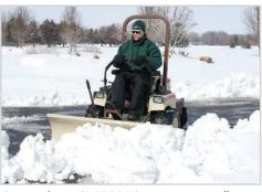
Multipurpose dozer blades offer unbelievable performance moving dirt, sand, gravel and snow. Blades operate straight ahead or 25 degrees left or right with manual pin positioning, and can be raised and lowered with hand or foot controls for easy operation, responsive control and timesaving efficiency.
