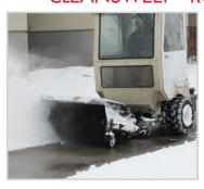
PTO-driven rotary brooms sweep dirt and debris, and clean up to 8 inches of snow. Only ½-¾-throttle is necessary for optimum efficiency. Fixedangle models sweep at a 25-degree angle to the right.
