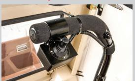
The optional Snow Performance Package increases productivity with on-the-go command of the implement. The joystick control, conveniently mounted to the steering lever, infinitely adjusts angles and height without leaving the operator's seat on the DriftBuster™ Snowthrower, CleanSweep<sup>™</sup> bidirectional rotary broom and the Little Bully™ PowerBlade™.
