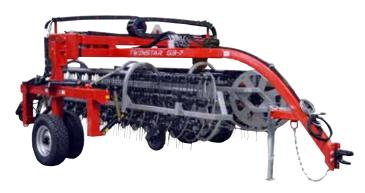
rocks, and debris) and has less leaf loss compared to traditional finger wheel and rotary rakes. Twinstar Generation 3 Hay Rakes are designed for functionality and longevity in today's demanding markets. Twinstar 7-Bar Rakes are available in 27 feet & 30 feet approximate raking widths for windrowers equipped with 12 foot to 18 foot headers.
