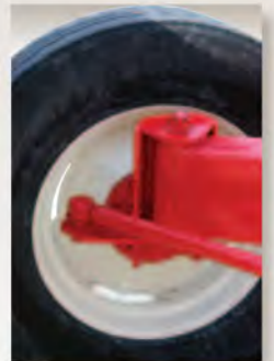
Heavy duty King Pins with taper roller bearings (all models)
