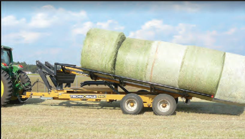
Pickup arm gently spins bale into position.
