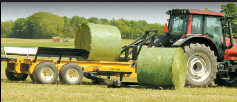
Pickup arm gently spins bale into position.
