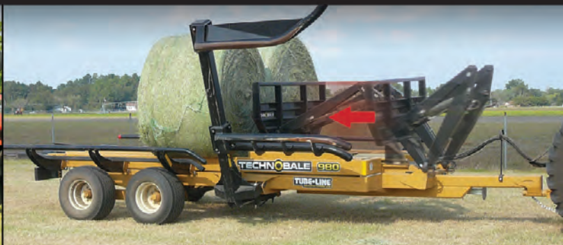
Scissor style pusher reduces cycle time.
