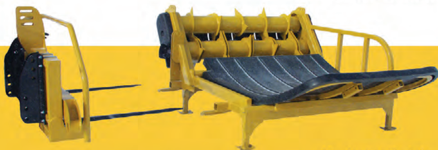
After loading the bale, the spear unit attaches by sliding into the frame, creating a single carrying unit.
