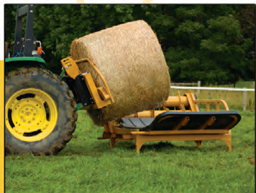
JAW COUPLER – automatically connects the feeding rotors with the hydraulic drive mounted on spear unit.
