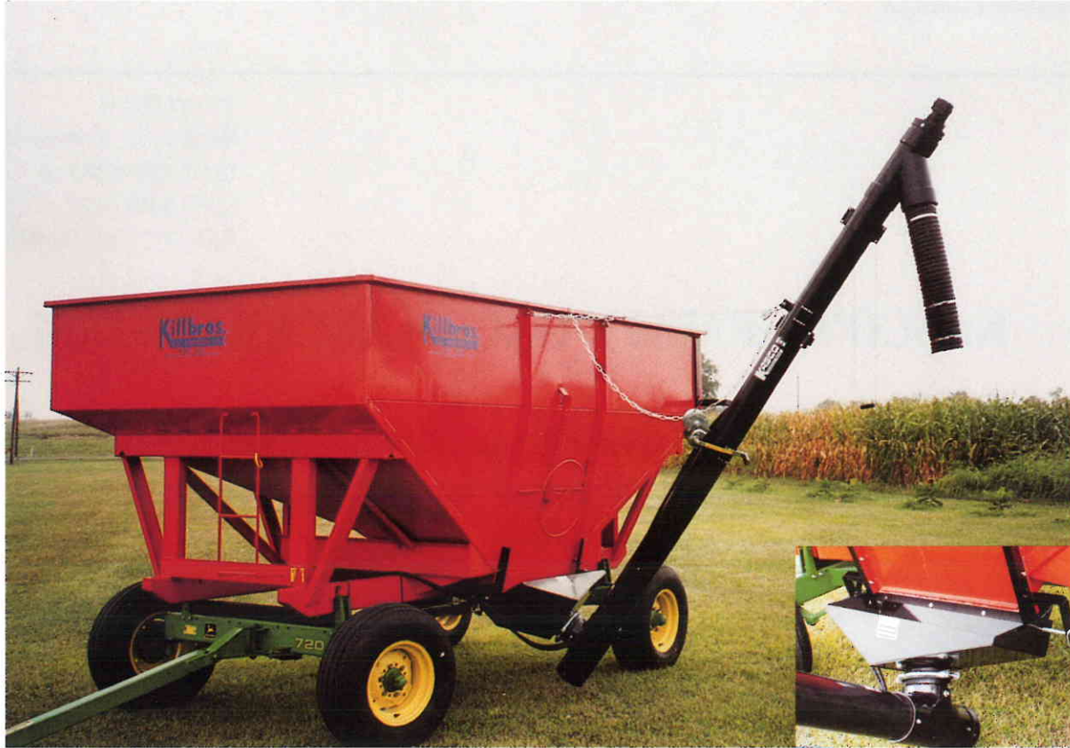
Showing Auger in Filling Position Innovative Hopper Design for Minimal Seed Damage
