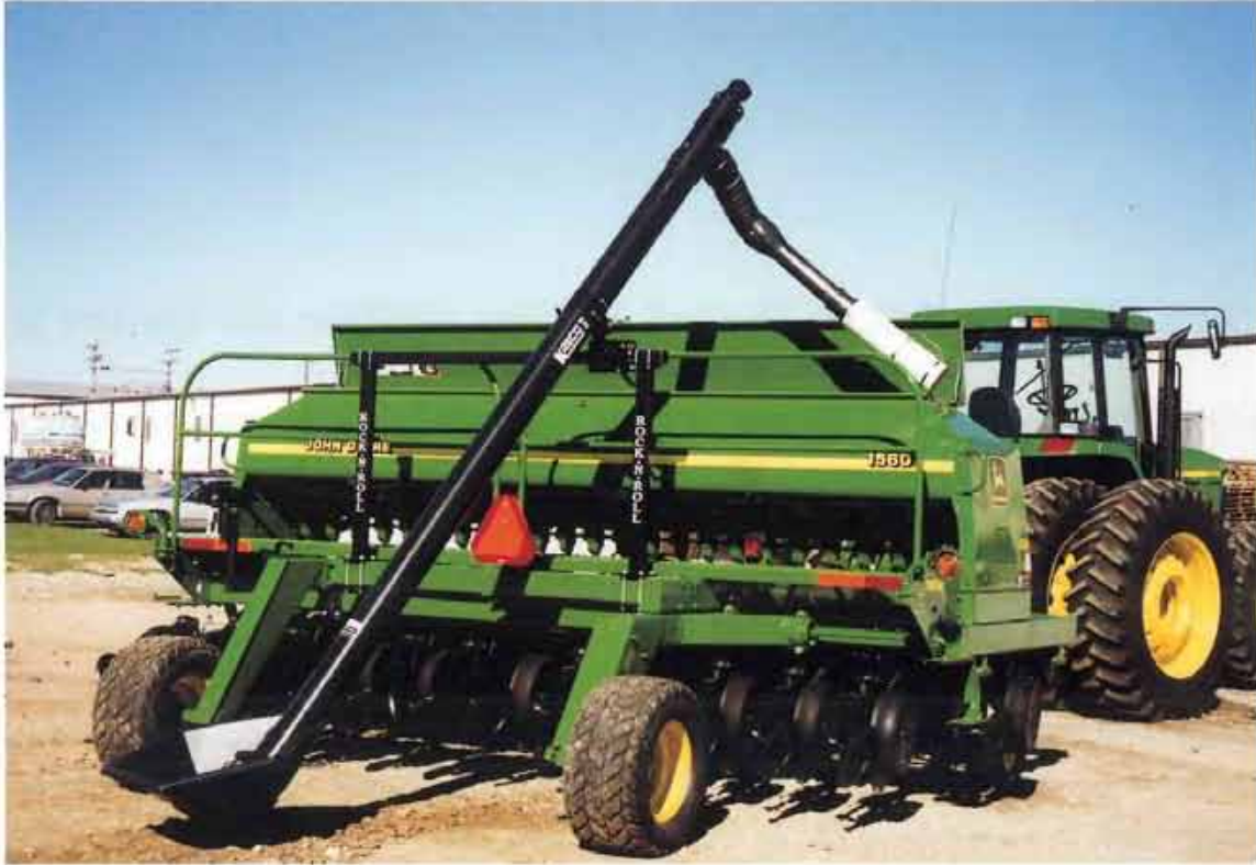
Showing Auger in Filling Position. Telescoping tube extends to reach end of hopper.
