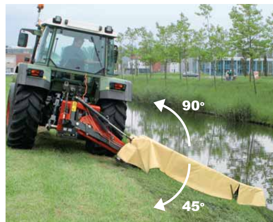
The CM mower bar can be operated at an angle of 90° vertical and 45° down slopes.
