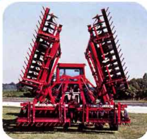
Folds with a big Massey disk for easy transport
