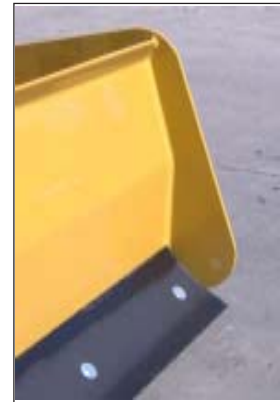
Side Plates Extended to Contain Soil when Back-Filling
