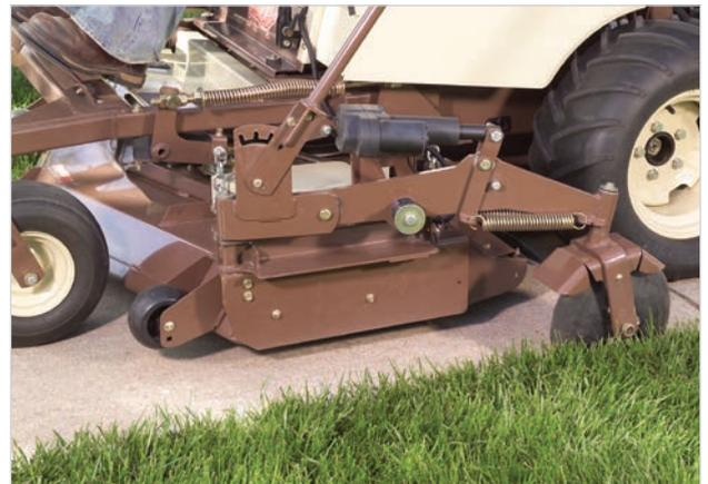
Left (trim side) mount for side and rear-discharge decks.
