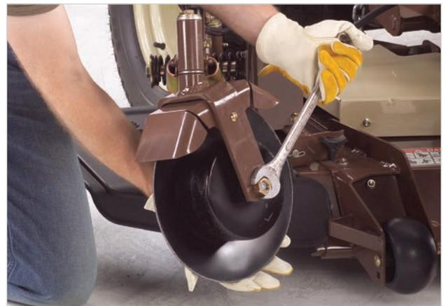
Reverse disc by removing one bolt to edge from the turf.
